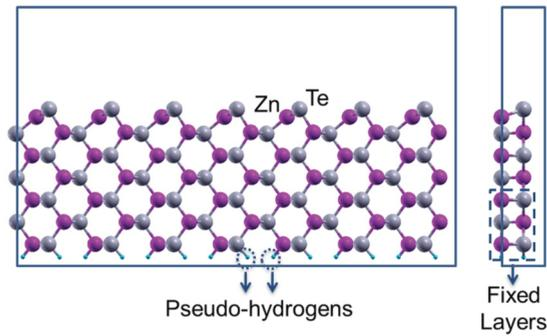
FIG. 4. (Color online) Two side views of the supercell used to simulate the (110) surface of ZnTe crystal. Lower surface of the slab is saturated by pseudo-hydrogen atoms to compensate effects of the artificial surface. During relaxation, lowest three layers of atoms are fixed at their bulk positions.
