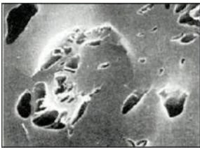
Magnified Pores in activated carbon
