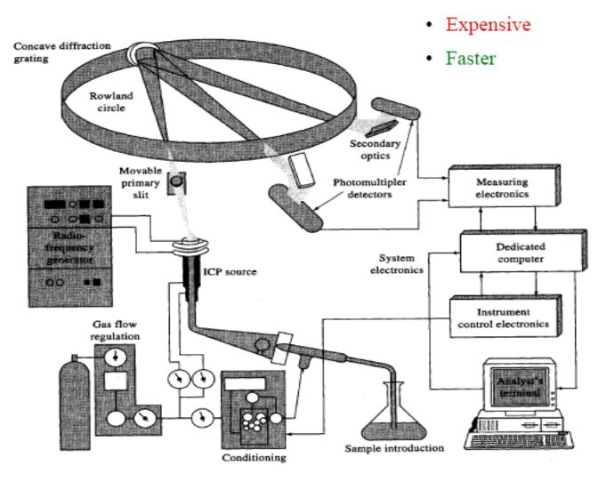
Since the atomic emission lines are very narrow, a high-resolution polychromator is needed to selectively monitor each emission line.
