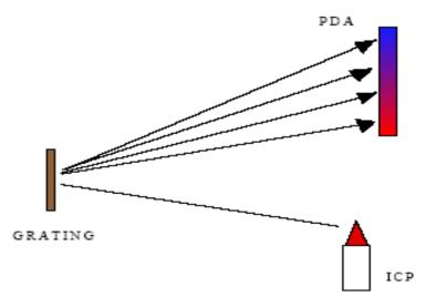
FIGURE 14. A PHOTODIODE ARRAY FOR SIMULTANEOUS ANALYSIS OF RADIATION.
