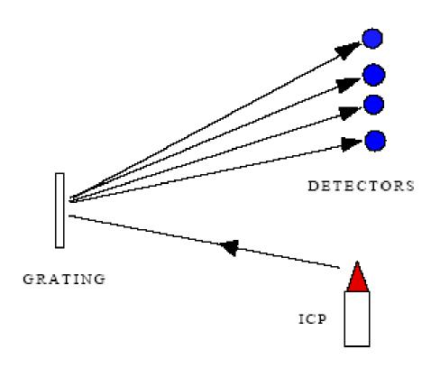
FIGURE 13. A POLYCHROMATOR FOR SIMULTANEOUS ANALYSIS OF RADIATION.
