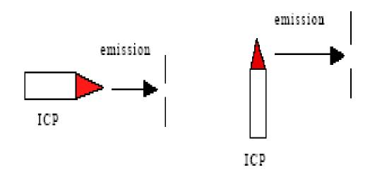
FIGURE 16. ICP TORCH POSITIONS INCLUDE A HORIZONTAL MOUNT (LEFT) AND THE MORE TRADITIONAL VERTICAL MOUNT (RIGHT).
