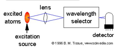
As in AA spectroscopy, the sample must be converted to free atoms, usually in a hightemperature excitation source
