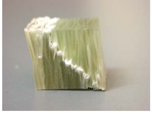
compression tested woven fabric S2-glass fiber reinforced vinyl ester composite
