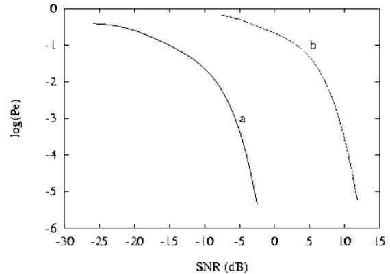
Figure 7. Comparison of the error probabilities of PISFE and matched filter type detectors, a: NCFSK, b: PISFE ( $\delta\omega = \pi / 100$ ,  $N=100$ ).
