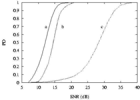
Figure 5. Comparison of the tone detection performance of PISFE, AR and periodogram type detectors, a: Periodogram b: AR c: PISFE ( $\omega = \pi/4$ ,  $P_F = 1E-4$ ,  $N=100$ , 500 noise realizations).
