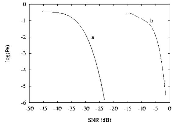
Figure 8. Comparison of the error probabilities of PISFE and matched filter type detectors, a: NCFSK, b: PISFE ( $\delta\omega = \pi / 100$ ,  $N=1000$ ).
