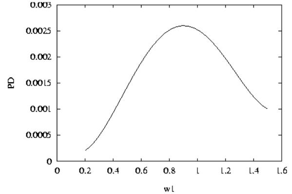
Figure 4. Variations of the tone detection performance of the PISFE detector versus tone frequency for constant detection band ( $\delta\omega=1.6E-4$ ,  $N=100$ ,  $\mu = 0$  dB).
