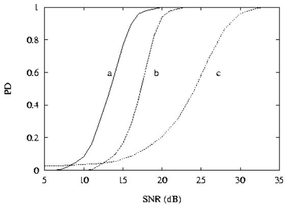
Figure 6. Comparison of the tone detection performance of PISFE, AR and periodogram type detectors, a: Periodogram b: AR c: PISFE ( $\omega = \pi/4$ ,  $P_F = 1E-4$ ,  $N=1000$ , 500 noise realizations).
