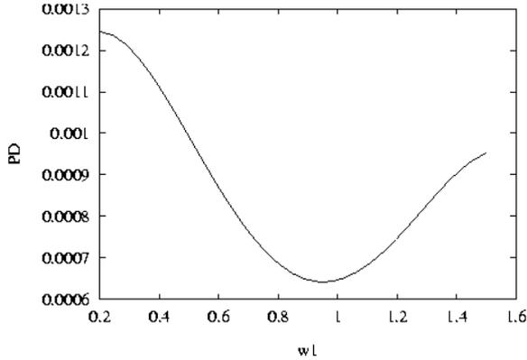
Figure 3. Variations of the tone detection performance of the PISFE detector versus tone frequency for constant probability of false alarm ( $P_F=1E-4$ ,  $N=100$ ,  $\mu = 0$  dB).
