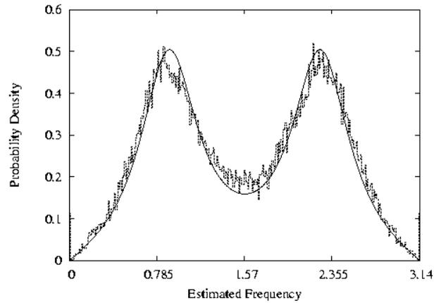
Figure 2. Pdf of the PHD frequency estimate for the  $H_0$  hypothesis versus frequency, solid line : analytic computation, histogram lines: histogram obtained by simulation ( $N=50$ , 100.000 noise realizations)
