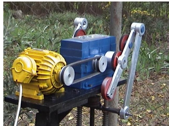
Fig. 4. A prototype of new constructive decision of a MDSRP with three stage package gear ( U_{\Sigma}=64 )
