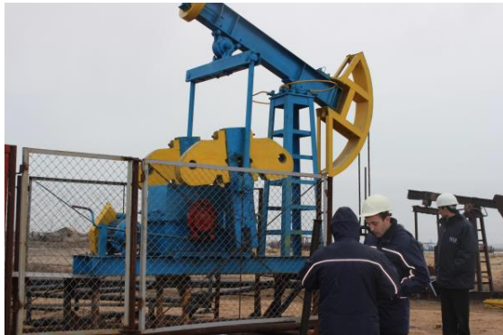
Fig. 5. Industrial test of sucker-rod pumps SKD 3-1.5-710 with three stage package gear ( U_{\Sigma}=64 ) in the oil fields of island "Pirallahy" near Baku
