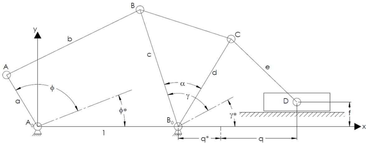
Fig. 1. Kinematic diagram of a Watt II mechanism
