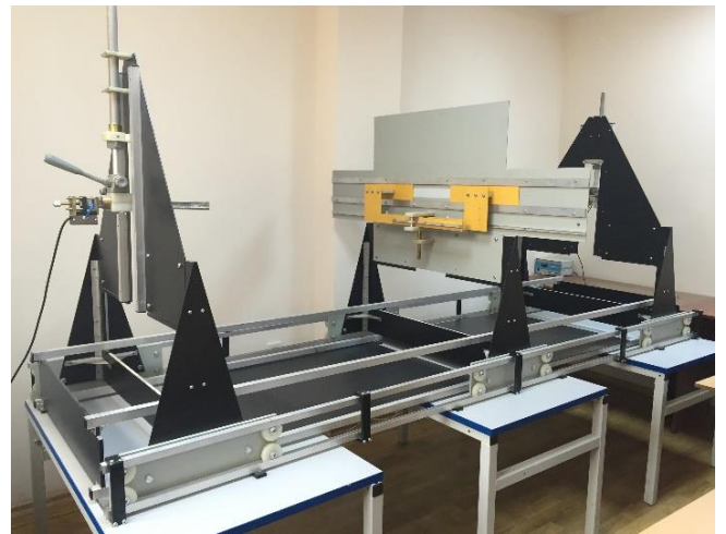
Figure 5. Space model of the experimental determination of orientation diagram
