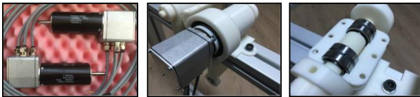
Fig. 7. Brushless Maxon Actuators and the Detail of the Passive Revolute Joint
